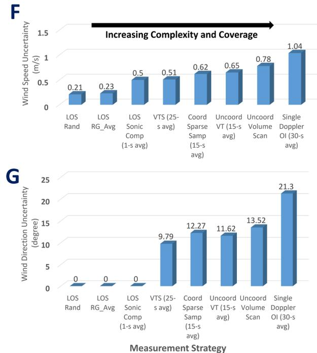
• Results demonstrate as Doppler wind lidar retrievals increase in complexity and coverage, uncertainty in both wind speed & direction increase [2] (Figures F & G)
