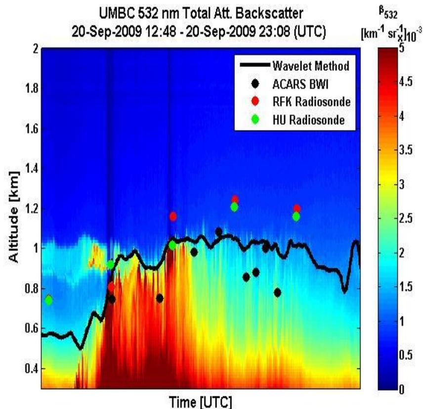
Lidar measurements helped to identify problems with automatic PBLH calculation from aircraft profiles (ACARS).
