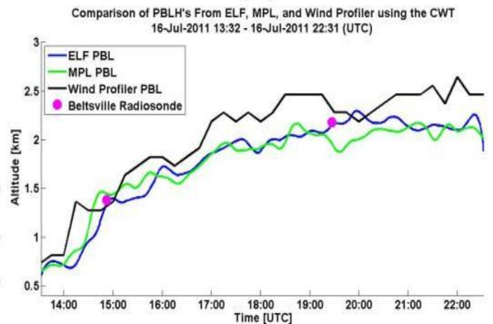
Lidar and radar wind profilers MLH from Covariance Wavelet Transform
